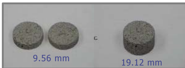
Figure 2 – (a) Two metal foam specimens. (b) A stack of the two specimens.
